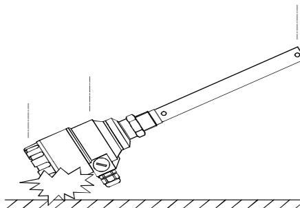
Avoid bending (single rod and coaxial probes) - Support the probe to avoid bending.
