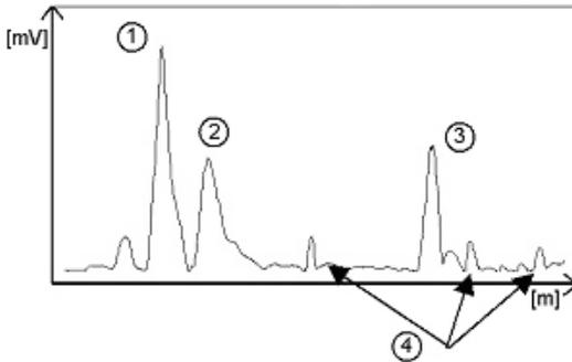
Even though the interference signals are very weak, the threshold should nevertheless be set to a value above these signals.
