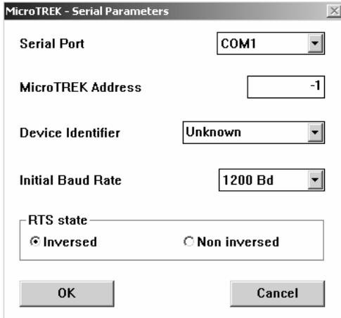
**Serial port** – The serial port allows the user to select a free serial port (COM 1 to 4) on the computer.
