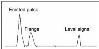
*Rod or cable probe with gain 1*
