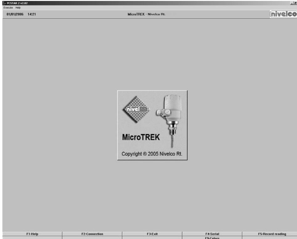
Define device interface: press F4 or left-click on "F4-Serial" at the bottom of the screen – to define the interface to which the device is to be connected.
