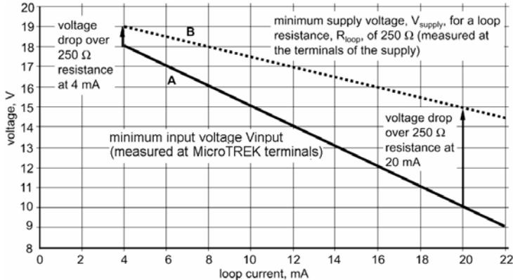
Line A = minimum voltage at the MicroTREK 2-wire terminals
