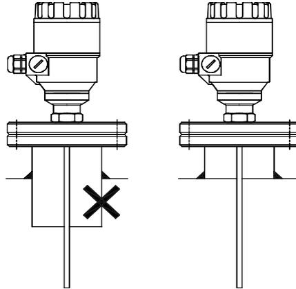
**X** Caution: Do not use nozzles that penetrate into the tank. This will disturb the emitted pulse.
