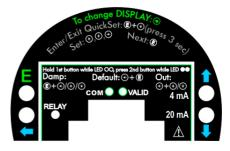
Procedure of programming: press button in the relevant sequence and check the state of the LED-s. Symbols for the states of the LED-s: ○ = LED is off, ● = LED is blinking, ● = LED is on, ● ● = LEDs are blinking alternatively ⊗ = Don't care
