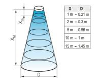
Diameters corresponding to 5° beam angle.
