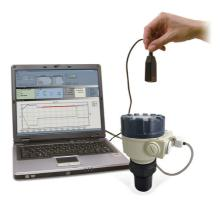
The IrDA adapter and the IrDA port of the device must be placed within a 5...10 cm distance and facing each other!
