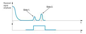
Some applications involve multiple (target + disturbing) echoes even within the measuring window. Basic echo selection will be done by the Quest + software automatically. This parameter only influences the echo selection within the measuring window.
