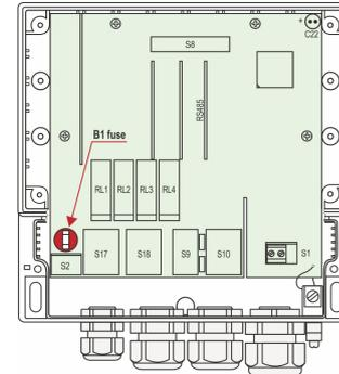
In order to change the fuse, loosen four nuts fastening the front panel, carefully tilt the front panel forward, such that the cable band is not under tension and replace the fuse.
