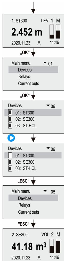
Once back in measurement mode the measured values of the devices found during detection are displayed one after another on the display. For the meanings of the captions on the display see 5.10 (Measurement mode). If the measured data of a given device are not needed temporarily, no needed to delete it from the list, it is enough to inactivate it in the following manner.
