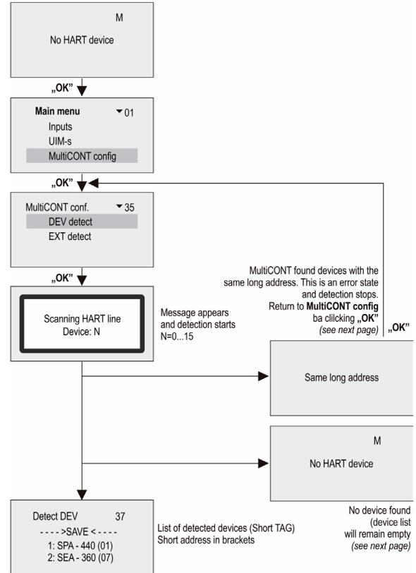
The **MultiCONT** detects devices by their Short address (that is why all short addresses must be unique within the system). However, it queries the devices by their Long address, which consists of the followings:
