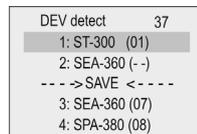
The Short TAG of responding units (either above or below →SAVE←) can be changed by selecting the device with **OK**. MultiCONT only handles units that are above →SAVE←.
