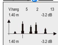
**Note!!** The displayed data corresponds to the moment of entering into the menu. The flashing echo is the one used by the transmitter to measure distance. To refresh the display press
