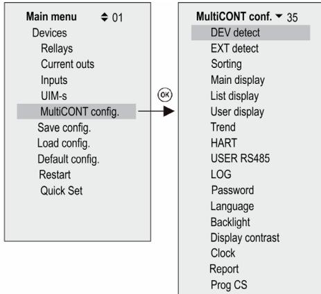
Navigate in the menu by using the and buttons, select items with the button.
