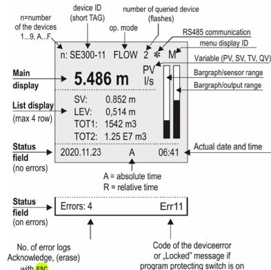
In this mode, it is possible to view the “Bar graph display”, the “User display” (Range, Double, Difference, Average see Main menu / MultiCONT config / User display – chapter 5.4) selected by the user, the relay-device and current output-device assignments, and also the error list, using and for selection. (See Appendix 5)
