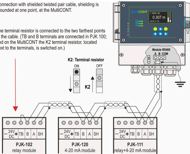
The most important rule is that the data transfer line has to be closed on both ends with a resistor, at points farthest from each other. The value of the termination resistor depends on the wave impedance of the connecting cable. The interface contains a 120  $\Omega$  terminal resistor, so please use a cable with appropriate impedance.
