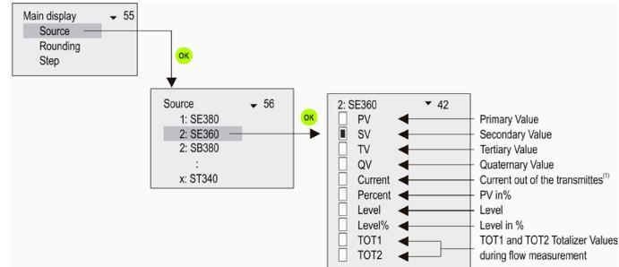
*(1) Output current changes only if there is just one device in the system, and its "Short Address" must be zero; otherwise, the current output is constant.*
