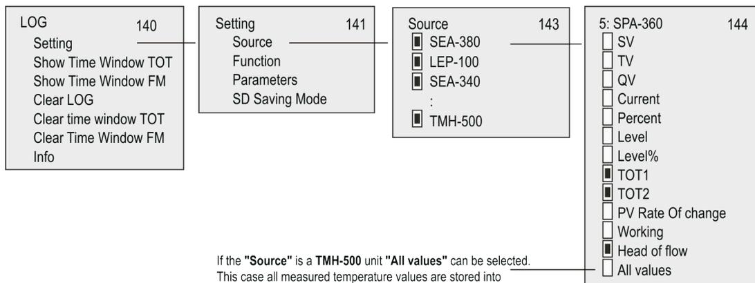
If the "Source" is a TMH-500 unit "All values" can be selected. This case all measured temperature values are stored into an additional row ("LT row") along with the standard logging entry ("LG row").
