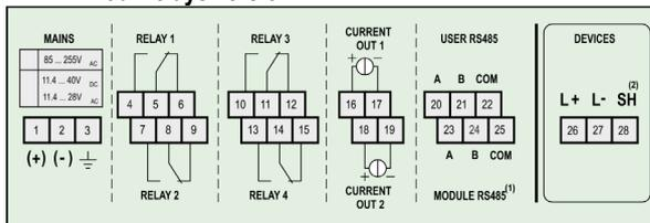
After removing the screws of the cover, cables can be connected. Use the appropriate wires for AC, DC, SELV, and mains.
