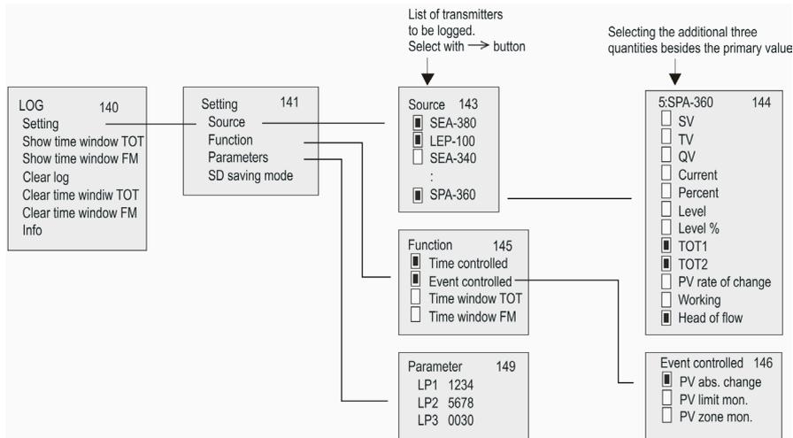
For using the trend logging function, the following data should be set:
