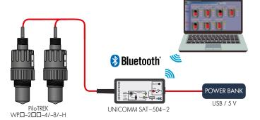
PiloTREK WP-200 level transmitter can be connected to a PC or cell phone via Bluetooth® wireless technology. WP $\square$ -2 $\square$  $\square$ -B/-E/-R devices can be connected directly, and WP $\square$ -2 $\square$  $\square$ -4/-8/-H devices can be connected using a UNICOMM SAT-504-2 modem.
