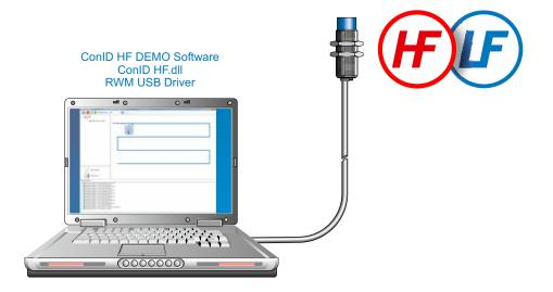
The default address of USB Read/Write Modules is 254.
