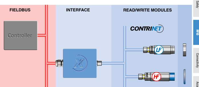
Communication between the RWM and any tags is provided by the modulation of a carrier. The frequency indicated for any RFID system is the frequency of its carrier.
